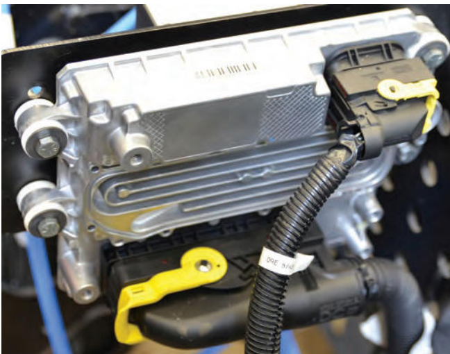
FIGURE 1-2 One of two modules used to manage the Detroit Diesel DD15 engine.
