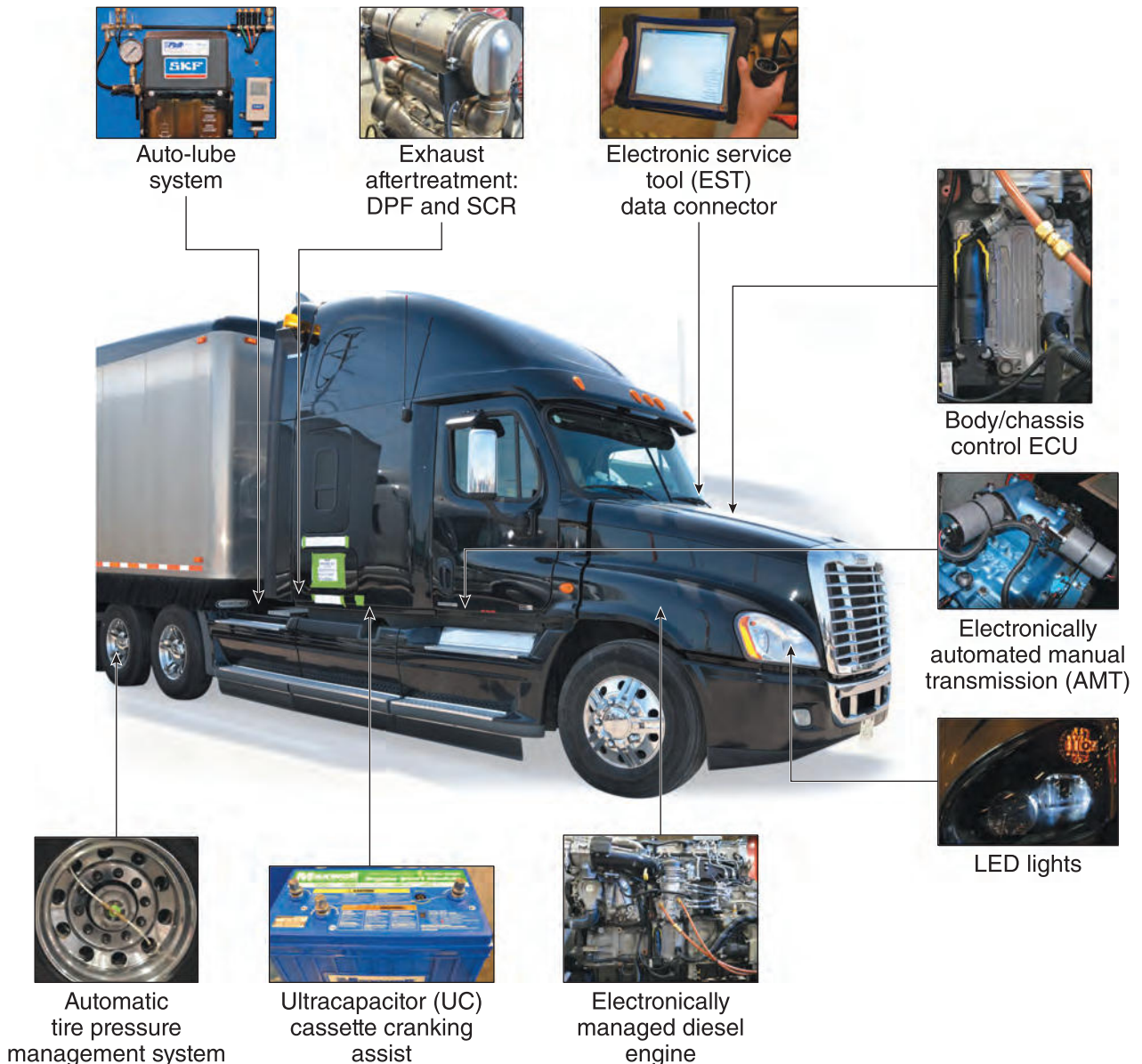
FIGURE 1-6 Multiplexed chassis computer-controlled systems used on a typical Class 8 truck.
